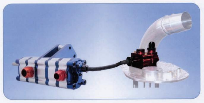
Raceline's new Cable-Driven Oil Pump was designed to remotely drive Waterman Racing Products' new cable-driven fuel pump. The advantage of driving the fuel pump from the rear of the oil pump is that the fuel pump is mounted on the fuel tank plate instead of on the side of the engine. As a result, damage to the fuel pump from major impacts, and the resulting fire, is virtually eliminated.
